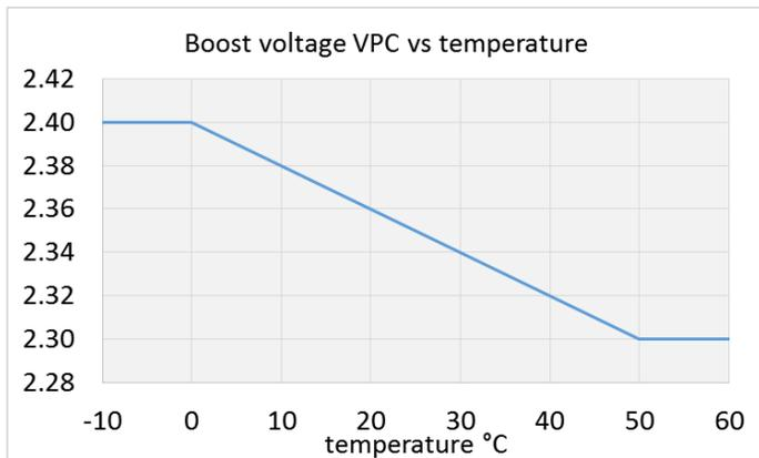
We also strongly recommend that the boost charge voltage shall be limited to 5 hours of duration. This is counted from the time the battery voltage reaches the boost voltage and the charging current starts to decrease.
