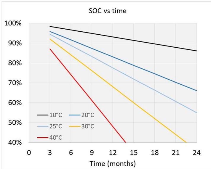
The 50% SOC limit corresponds to 12.2 V for a monobloc recharge before this limit is passed.
